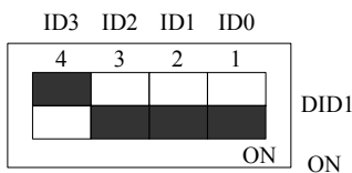
The above chart shows "0111", so it means that the physical ID is 7.
