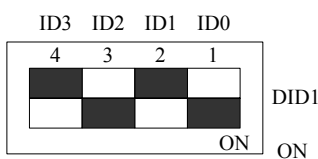
The above chart shows "0101", so it means that the physical ID is 5.
